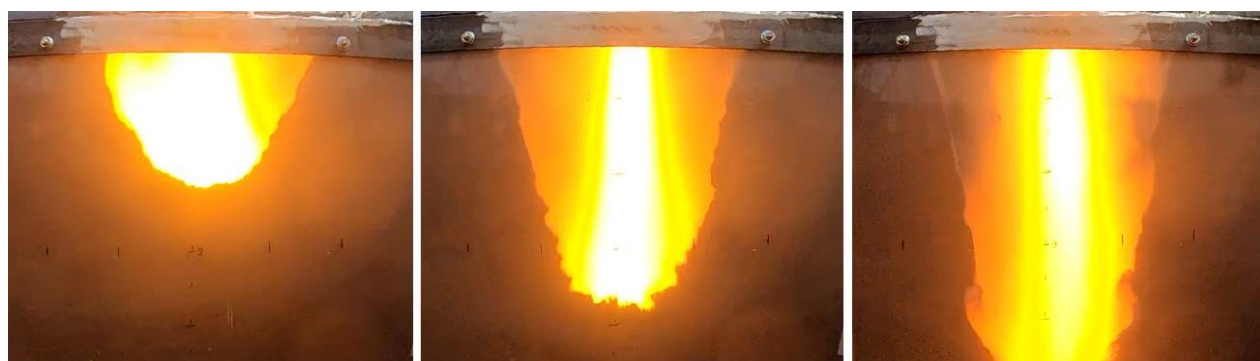
Deep Crater Formation Visible Through Split-View Window During Hot Fire Test (Masten Space Systems 2022)
