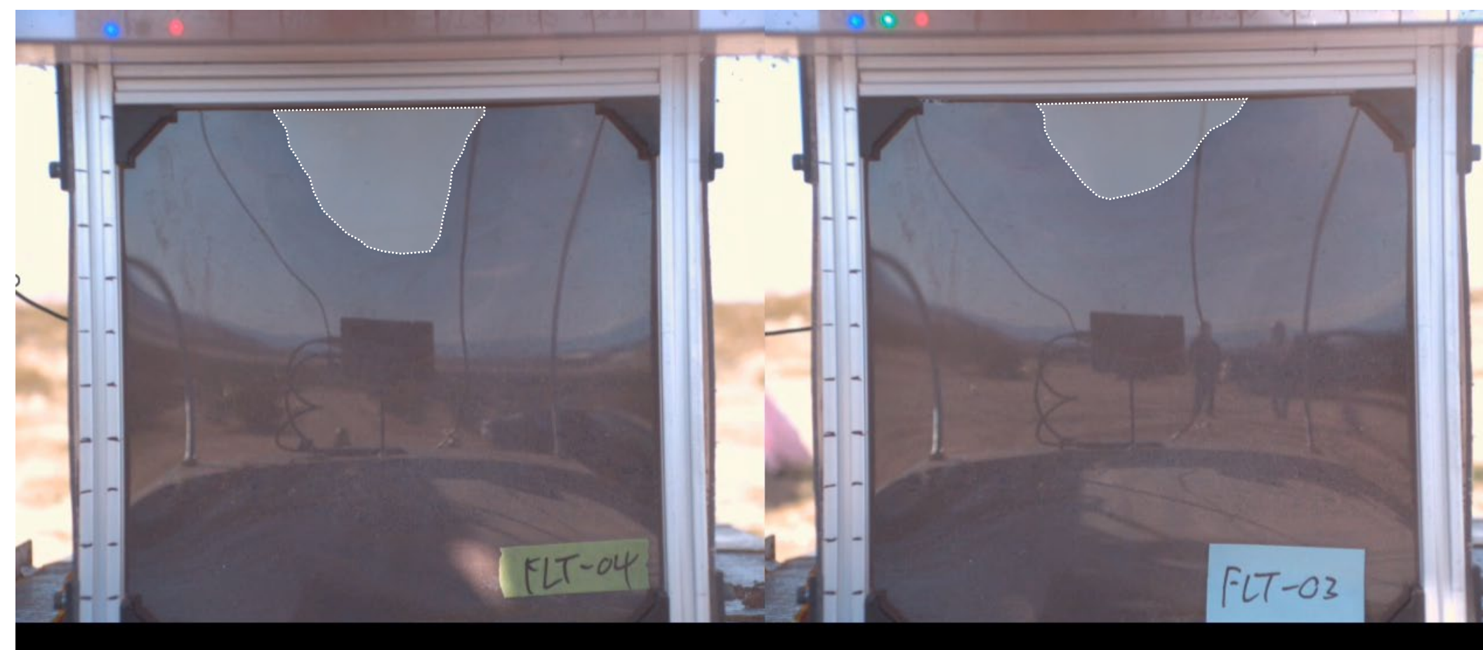
Crater Formation Comparison During Tests (Highlighted); Test No. FLT-04 at Reduced Gravity (Left); Test No. FLT-03 at 1-g Gravity (Right)
